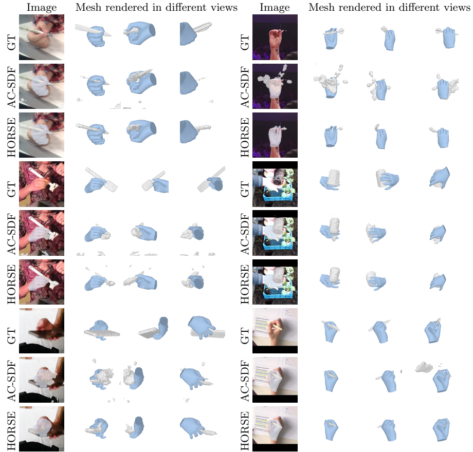
Fig. C: Mesh visualizations on MOW object generalization split. We show the object mesh projected onto the image and rendered in different views for our HORSE model and compare with the AC-SDF model trained on ObMan dataset with 3D supervision (best baseline model). We also show the ground truth (GT) object model. We observe that our model is able to predict the object shape more accurately than AC-SDF which often reconstructs smaller and disconnected shapes.
