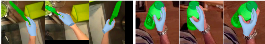
Fig. 4: VISOR visualizations. Using existing hand pose estimation techniques [54], we are able to track the objects in relation to hands through time in in-the-wild videos. We visualize these tracks along with object masks from the VISOR dataset [13]. This form of data, where objects move rigidly relative to hands, is used to train our model to learn 3D shape of hand-held objects.
