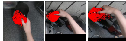
Fig. 7: Sampled points do not cover the entire object if hand pose is inaccurate.
