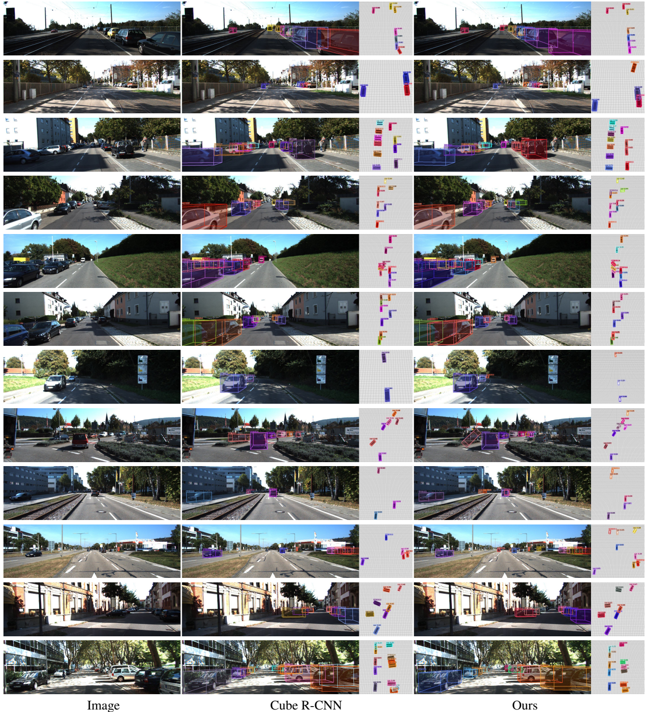
Figure 4. 3D Object Detection on KITTI [5] . We show the 3D bounding box predictions on Cars category for Cube R-CNN [2] and our model (Cube R-CNN + KPE), both in image space and in top-down view. Our model predicts better 3D bounding boxes, as evident by fewer collisions ( i.e. intersections between car bounding boxes) and missed detections.
